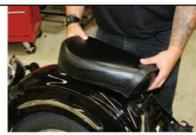
With the main section set aside, slide the passenger pillion forward to remove it from the Road Star.
