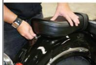
Using a 10mm Allen wrench, loosen and remove the fastener that holds the passenger seat in place.
