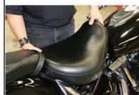
Turning the ignition key allows you to lift the front portion of the Yamaha seat free of its mounts.
