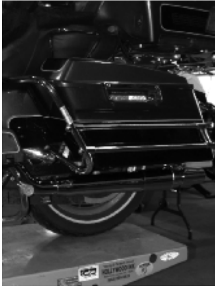
18 Here's the left side of the bike with the new Thunderheader system installed.
