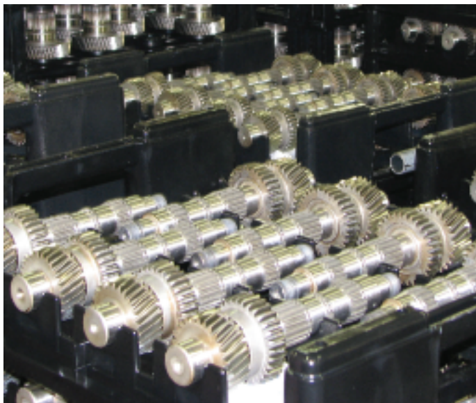
The 2007 H-D six-speed tranny uses both spur-(straight-cut) and helical-cut gears, as you can see on these tranny components at a H-D manufacturing facility.
