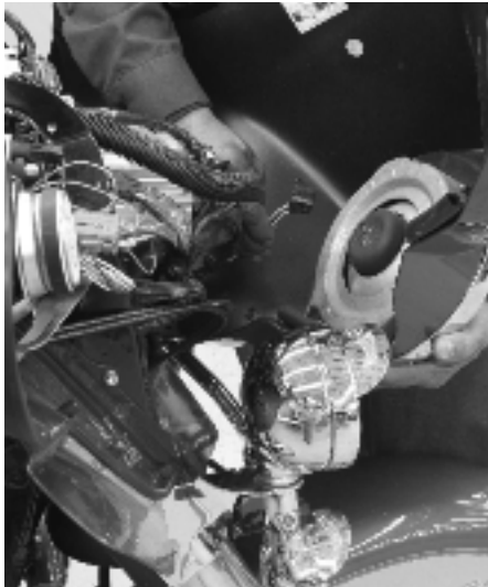
11 Charlie plugs in the headlight before reattaching the fairing.
