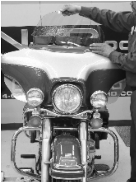
12 The windshield can now be moved into place and reattached using the three stock bolts along the top of the fairing and a T27 Torx drive. AIM
