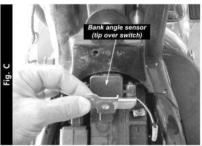
6 Unbolt and move the bank angle (tip over) sensor out of the way (Fig. C).
