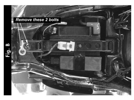
5 Remove the battery/ECU hold down bracket (Fig. B).
