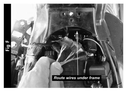
10 Continue routing the wires from the PCIII under the frame near the lower fuel tank mount and go up to the throttle body area (Fig. F).
