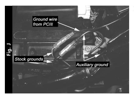
19 Disconnect the stock ground wire (black with yellow stripe) from the negative battery lead. Plug the wire with the male bullet connector from the PCIII into the female end of the stock connector and plug the female end of the auxiliary ground wire into the male end of the stock connector (Fig. J).
