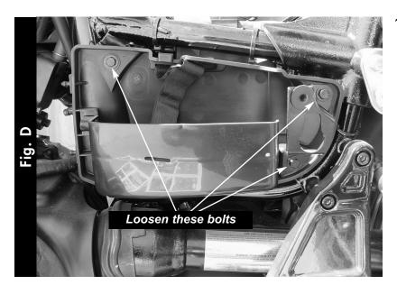
Loosen the bolts holding the plastic tray on the left side of the bike (under the left side cover) (Fig. D).
