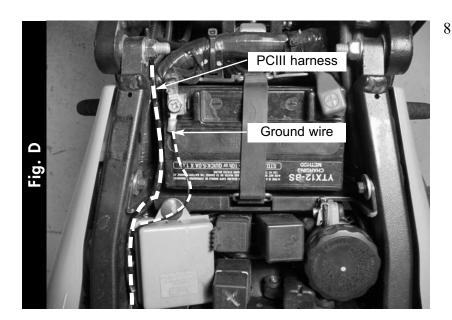
Attach the ground wire from the PCIII to the negative side of the battery (Fig. D).
