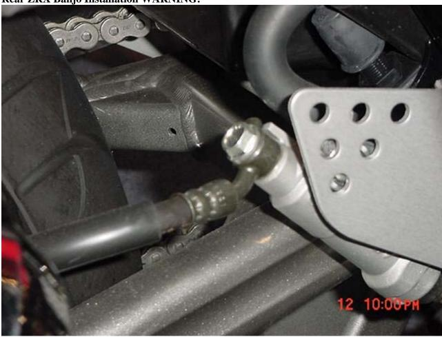
When installing the rear brake line on your ZRX1100 or 1200, please make sure the rear master cylinder banjo is facing the same way your stock banjo was before. Failure to do so will break the Galfer banjo, and cause the brake fluid to leak. Please remember not to torque the banjos over 15 foot lbs.
