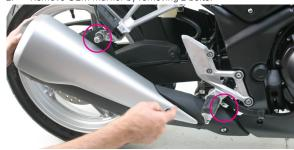
Apply a thin layer of anti-seize to TBR slip tube outlet and connect to Tarmac muffler using supplied hook springs. Loosely install barrel clamp onto slip tube inlet.
