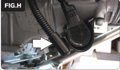
12 Unplug the stock O2 sensor from the main wiring harness on the left hand side as shown in Figure G.
