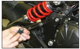
4. Remove muffler mounting hardware.
