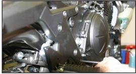
Slide the (rubber-lined) muffler clamp over the muffler canister and install header on bike using supplied flange bolt and nut on muffler clamp.
