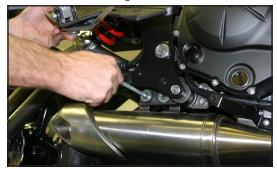
Remove header nuts from cylinder head and remove header assembly.
