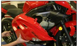
Remove the right foot rest assembly to access muffler mounting bolts.
