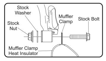
4. Standing at the back of the motorcycle, check for proper alignment of the muffler and adjust if necessary.
