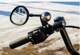
The Kustom Semisphere Mount attaches to your stock controls. Remove 2 bolts from the controls, line up the mount, and use the included hardware to tighten. Follow factory specs. Tools needed: T30 torx and 4mm allen wrench.
