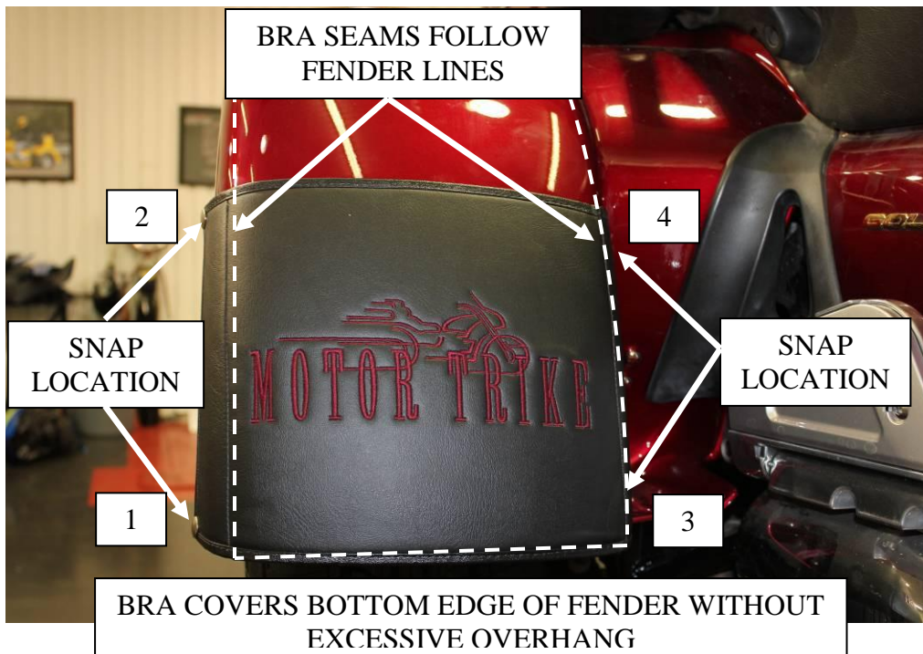
FIGURE 1: INSTALLATION FEATURES OF THE FENDER BRAS
