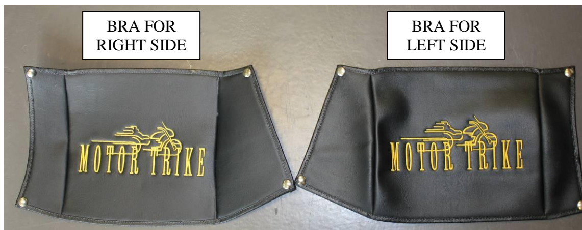
FIGURE 2: FENDER BRA ORIENTATION
