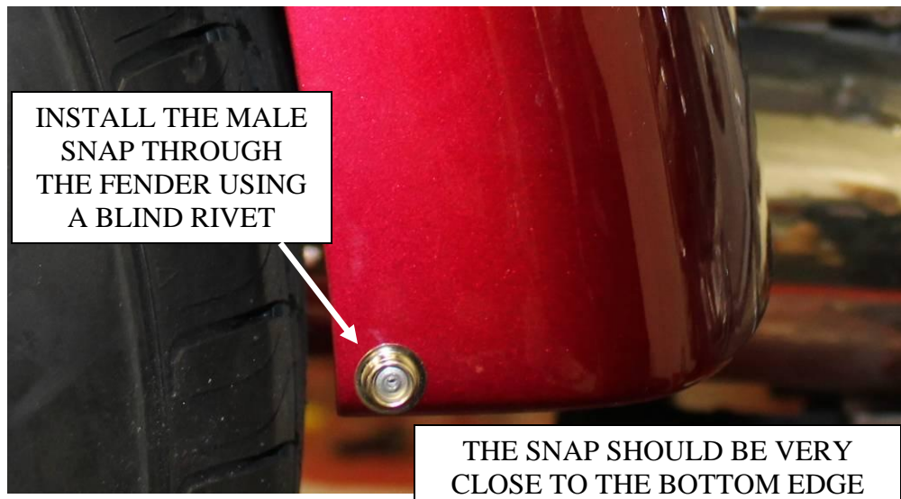
FIGURE 5: SNAP 1 INSTALLED ON FENDER
