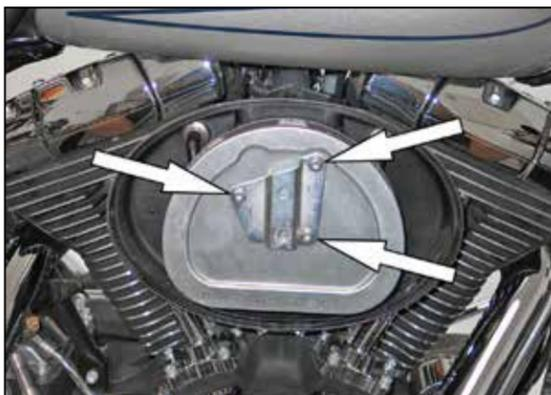
3. Remove the three bolts that secure the air filter to the filter base and then remove the air filter along with the crankcase breather tubes.
