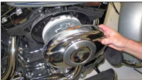
2. Remove the bolt that secures the bonnet to the filter assembly and then remove the bonnet from the vehicle.
