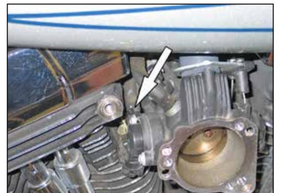
6. Using the provided tie wrap, secure the wiring pig tail to the throttle body wiring harness.
