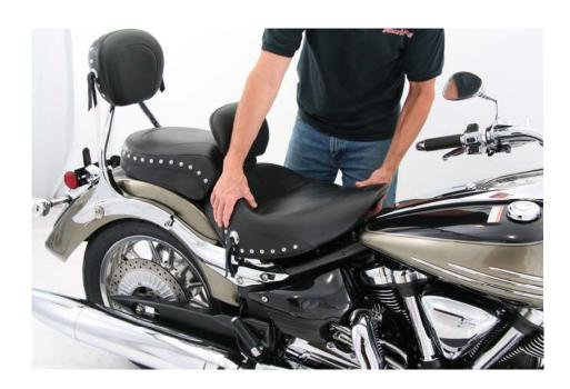
3. Align the nose bracket with the frame receiver and push down until a click is heard, signifying the solo is latched into position. Ensure this bracket is firmly engaged before riding.
