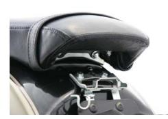
3. Lift the front of the passenger seat and slide forward to remove the solo seat.
