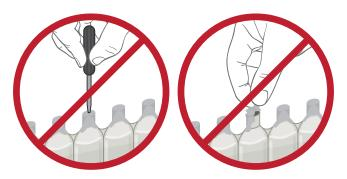
Do not puncture the foil seal or remove it prior to filling a dry AGM battery.
