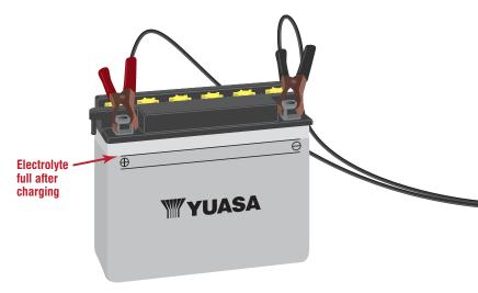
Make sure that the acid level is to the upper mark after the battery is initially charged. If the level is low fill with electrolyte.
