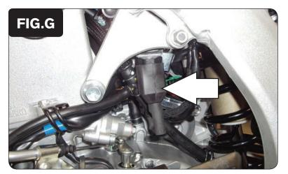
Pull back on the rubber boot covering the Throttle Position Sensor connector to expose the stock TPS wires (Fig. G).
