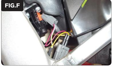
Plug the pair of PCV wiring harness leads with YELLOW colored wires in-line of the secondary injector and stock wiring harness (Fig. F).
