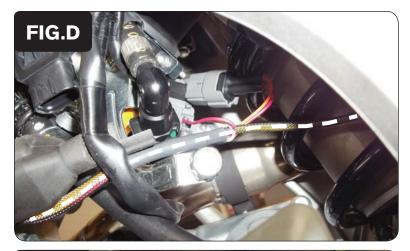
Plug the pair of PCV wiring harness leads with ORANGE colored wires in-line of the primary injector and stock wiring harness (Fig. D).
