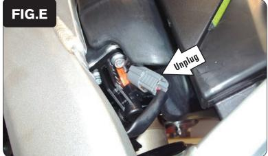
6 Locate and unplug the Secondary Fuel Injector (Fig. E).
