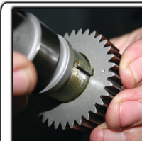
Line up gear with camshaft
