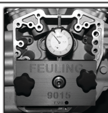
Feuling Runout Measuring Tool #9015
