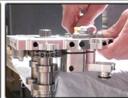
Bolt oil pump to camplate finger tight DO NOT use loctite or hardening compound
