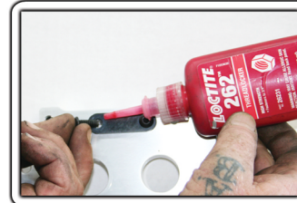
Apply Loctite to block off plate bolts
