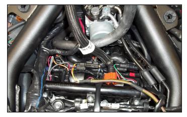
13 Plug the PCV harness in-line of the stock wiring Harness and injectors
