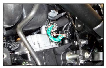
12 Unplug the stock wiring harness from each injector.
