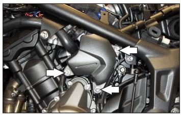
9 Unplug the Crank Position Sensor connector.
