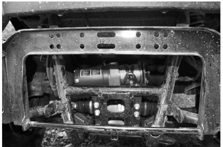
*Figure 2 Place Winch Inside The UTV Frame*
