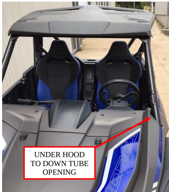
Figure 10: Chassis harness routing under hood to opening.
