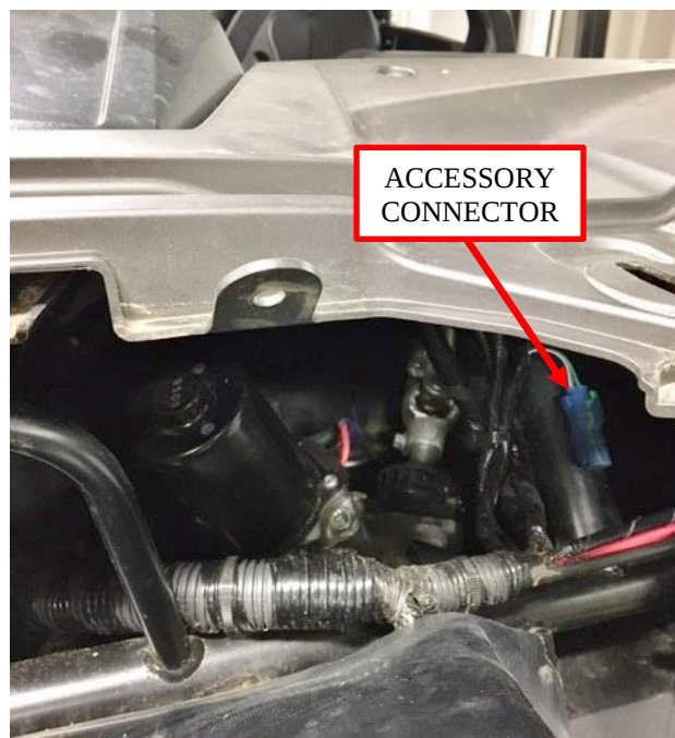
Figure 8: Factory accessory connector location.
