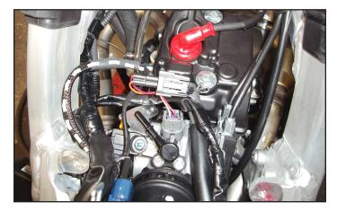
7 Unplug the Throttle Position Sensor at the left side of the throttle body.
