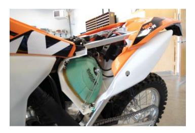
2 Remove the left side panel covering the air filter.
