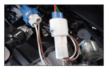
15 Attach the PC6 connectors to the stock CPS connectors.
