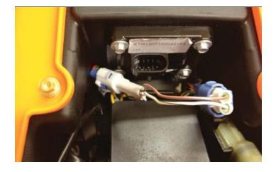
6 Plug the PC6 wiring harness in-line of the stock CPS connectors.
