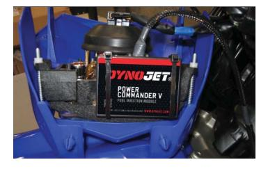
4 Attach the PC6 to the bottom of the headlight using the supplied zip ties.
