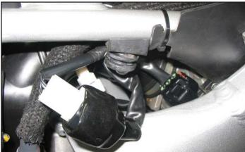
11 Plug the PC6 connectors in-line of the stock TPS and wiring harness.
