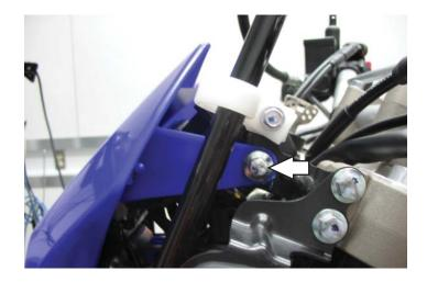
3 Remove the headlight by removing the bolt shown on both sides.
