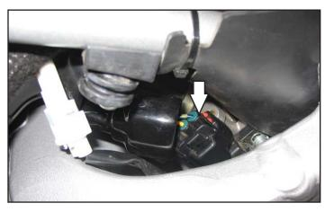
9 Locate the Throttle Position Sensor connector on the right hand side of the throttle body.
