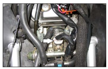
8 Plug the PC6 connectors in-line of the stock wiring harness and injector.
