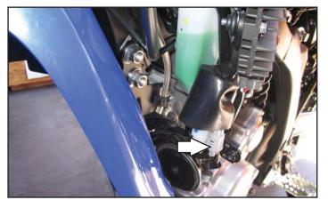
12 Locate the 2-pin GREY connector under the left hand radiator cover.
