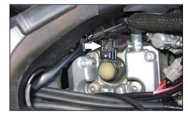
16 Plug the PC6 in-line of the stock wiring harness and coil stick.
