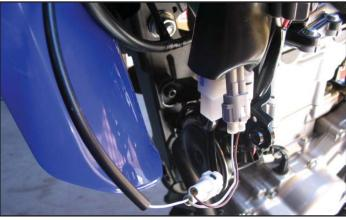
14 Plug the WHITE connectors from the PC6 in-line of the stock wiring harness and crank pickup coil sensor.
