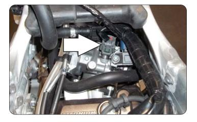
5 Locate and unplug the stock wiring harness from the fuel injector on top of the bike's throttle body.
