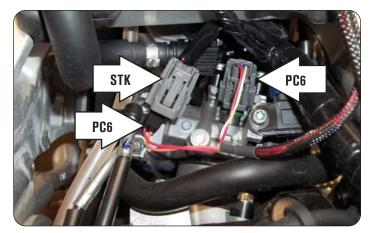
7 Locate and unplug the stock wiring harness from the bike's Throttle Position Sensor.
