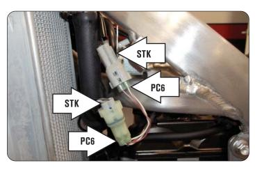
10 Plug the PC6 wiring harness in-line of the stock wiring harness and CPS.
