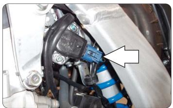
8 Plug the PC6 wiring harness in-line of the TPS and the stock wiring harness.
