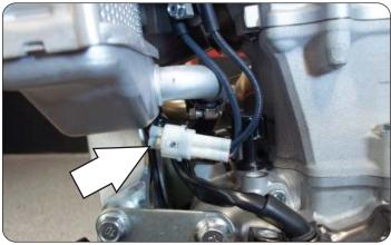
11 Locate and unplug the stock wiring harness from the bike's Ignition Coil.
