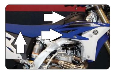
1 Remove the seat, the radiator side covers, and the fuel tank.
