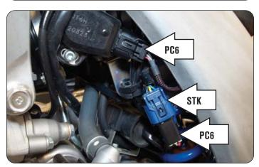
9 Locate and unplug the stock wiring harness from the bike's Crank Position Sensor.
