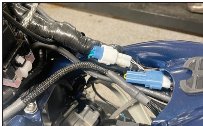
CONNECT TO CRANK POSITION SENSOR
