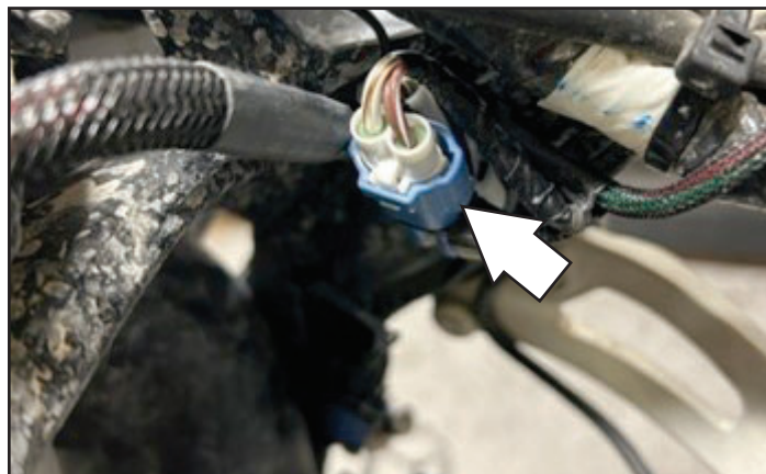
UNPLUG CRANK POSITION SENSOR
