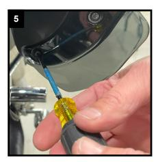
Remove left and right speaker grills. The speaker grills are held in place by clips. Remove by pushing outwards from the inside of the speaker grills shown in Figure 6.
