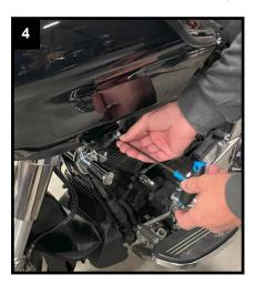
6. Remove left and right side lower air deflector T25 Torx bolts shown in **Figure 5**.
