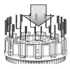
**Note:** If the basket sleeves fall forward while installing the clutch pack, use a pick to push the basket sleeves back into place.
