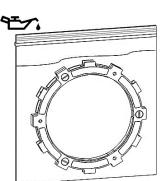
2.Install all the Rekluse basket sleeves into the basket slots. Make sure the bottom of the sleeve is facing down, and the sleeve tabs sit against the inside of the basket. See pictures for reference.
