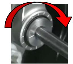
C) Once you have found the starting point, note the position of the hex key using the tick marks on the slave cylinder housing and the small etch mark located on the screw. You will begin here to adjust the installed gap.
