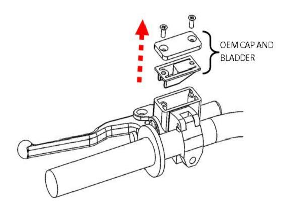
3. Top off the master cylinder with the recommended clutch fluid until it is 75% full.
