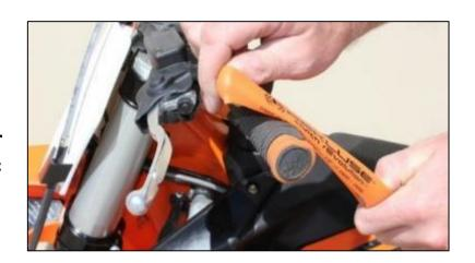
c) While holding the top end of the rubber band against the handlebar, stretch the band downward, then loop it through itself.
