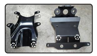
5. Re-install stock tail light onto tail light bracket.
