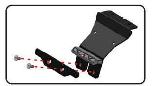
Note: M6X10BHS, button head screws will be used to secure the license plate to FE-LP-BKT, license plate bracket. 6MMLN-SS, nylon lock nuts and 6MMWASHER-SS, washers are for the bottom license plate holes.
