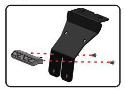
Install FE-LP-BKT, license plate bracket onto 13710-FEBKT-4, fender eliminator bracket using M6X12FS, flat head screws.
