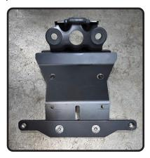
4. Install 13710-FEBKT-4, fender eliminator bracket on top of stock rear fender reinforcement bracket using M6X14BHS, 6mm screws.
