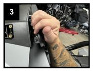
5. Remove vent cover by lifting up and out and do not lose the rubber windshield posts. Shown in **Figures 4 & 5.**
