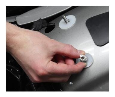
2. Engage the nose bracket into the frame. Push it forward until the hole in the rear bracket is aligned with the threaded fender nut. If needed, a firm downward punch or chop to the nose of the seat will push the seat closer to the tank dash.
