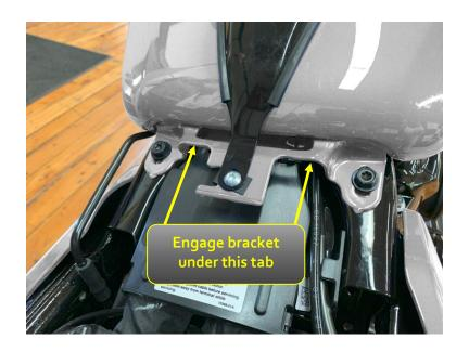
3. Secure rear bracket with the stock plastic washer and  $\frac{1}{4}$ "-20 thumb screw.
