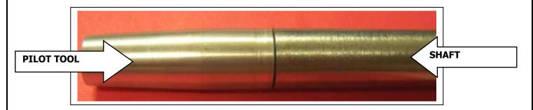
**7**. Remove the Harley shaft a little at a time while simultaneously from the opposite side start inserting the Mad Dog shaft from the pilot tool side.
