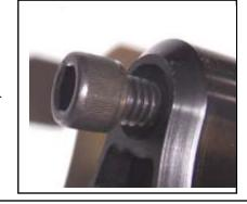
11. Shaft must be flush or no more than .030" inside spacer for proper preload. See arrows
