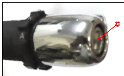
A — Friction Nut & Grub Screw B — Kaoko bar-end Body C — OEM bar-end weight D — Kaoko M12x90 Screw
