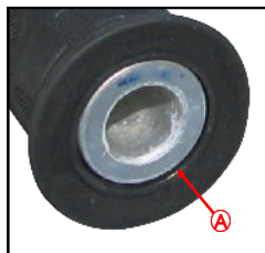
A — Throttle Sleeve (when bar-end is removed)
