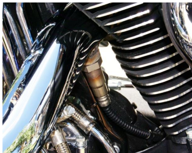
Typical Rear Sensor Installation
