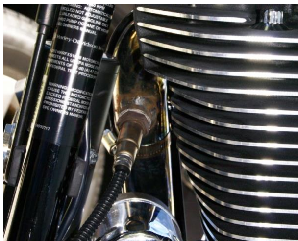
Typical Front Sensor Installation
